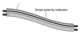
Your cables may also be marked for directionality with arrows. In this case, the arrows should always point in the direction of signal flow towards the speakers.
