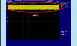
Example of waveform in check ② Voltage scale : 1.0V/div Time scale : 1s/div
