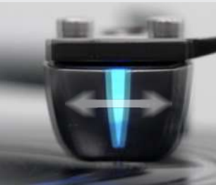
There is eccentricity: Cartridge is forced to sway
